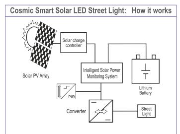
Solar PV module converts sunlight into DC power and this is stored in the Lithium battery. Solar charger optimizes solar charging and prevents battery over charge / deep discharge. Converter converts DC power into light. PIR motion sensor controls LED light brightness. The system shall work on solar power, without grid power.
