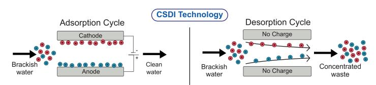
Our patented technology of capacitive deionization works when electricity is applied to the electrode, ions of opposite charge pass through the ion exchange electrode and move to the surface of the electrode and are electrically adsorbed
